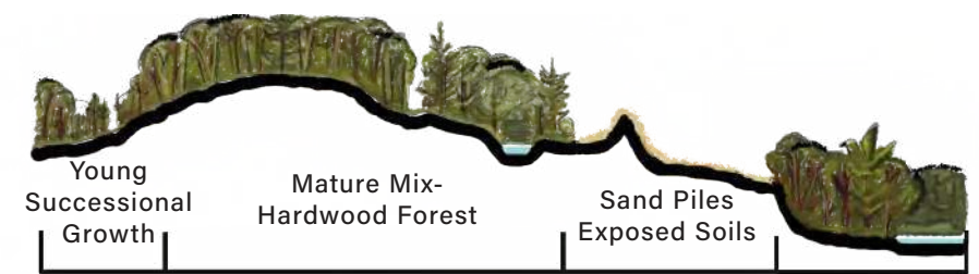
Section B-B' shows the change in elevation across the site from the high point to the low point. Exaggerating the vertical axis helps reveal the natural depressions where vernal pools form as well as the dramatic presence of the sand piles in the center of the property.
